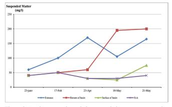
Figure 8. Spatio-temporal trends in suspended matter concentration of water samples collected from four locations of treatment station during study period.
