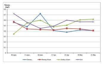
Figure 11. Spatio-temporal trends of nitrate ions concentration in water samples collected from four locations of treatment station during study period.
