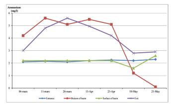
Figure 10. Spatio-temporal trends of ammonium concentration in water samples collected from four locations of treatment station during study period.
