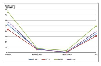
Figure 14. Spatio-temporal trends of number of fecal coliforms in water samples collected from four locations of treatment station during study period.
