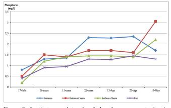
Figure 9. Spatio-temporal trends of phosphorus concentration in water samples collected from four locations of treatment station during study period.
